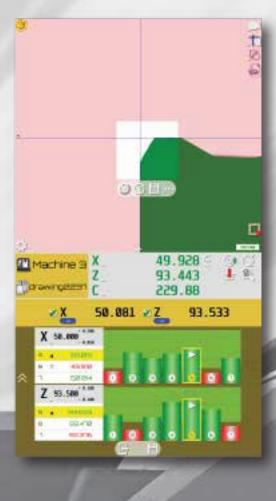
Elbo Controlli NIKKEN has developed a system that adapts the peripheral rotation speed of the tool based on the maximum diameter to be measured: the constant peripheral speed avoids the introduction of errors, whether you are measuring a 2 mm diameter tool or a 200 mm one.
